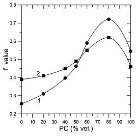
**Figure 1.** *f* values vs PC content calculated with eq 1 by using the luminophore quenching couple  $Ru(bpy)_3^{2+}/MV^{2+}$  (1) or pyrene/C-153 (2).
