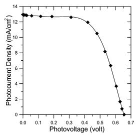
**Figure 3.** I-V curve for an optimized DSSC. ff = 0.66.
