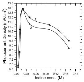
**Figure 4.**  $I_{sc}$  curve vs iodine concentration for an electrolyte containing all components (1) and without NMBI (2).
