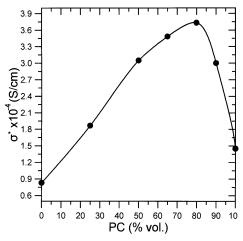
**Figure 2.** Dark dc conductivity values for the SiO<sub>2</sub>/Triton/PC/I<sub>3</sub>-/I<sup>-</sup> electrolyte at varying PC content.
